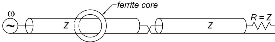
Show that if  $m$  intermediate segments of impedance  $Z_I = 2Z_P$  are used instead two, shorting the inner and outer conductors of adjacent cables at their output ends, the resulting transmission-line transformer makes a  $1 : m^2$  impedance match (1:m voltage transformer).
