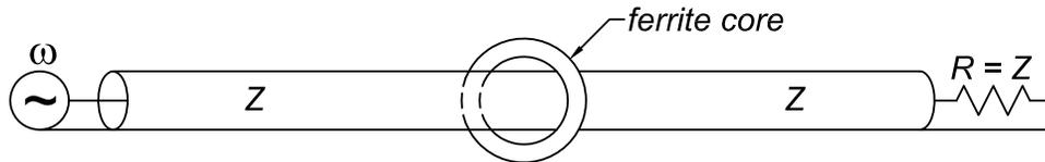
A more nontrivial variant is obtained if a second coaxial cable is attached to the first (the one that passes through the ferrite core), with the conductors of the two cables cross connected as shown below. In this case we obtain a 1:1 inverting transmission-line transformer.
