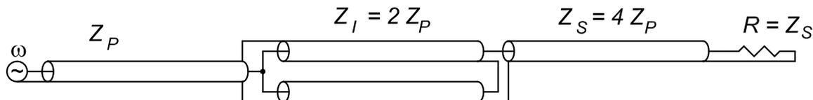
Verify the desired functionality of this circuit, supposing that the intermediate segments of transmission lines are long enough that TEM waves propagate in them. This has the effect that the voltages at the two ends of these segments are isolated from one another, because the integral  $\int \mathbf{E} \cdot d\mathbf{l}$  along the line vanishes for a TEM mode.
