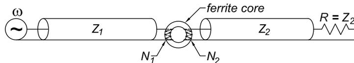
To maximize the flux linkage in practice, it is advantageous to wind the two coils around a ring or “core” of a high-permeability magnetic material, such as a ferrite. See, for example, [7]. However, the performance of magnetic materials is limited at very high frequencies, so a ferrite-based, flux-linked, impedance-matching transformer has only a finite bandwidth.
