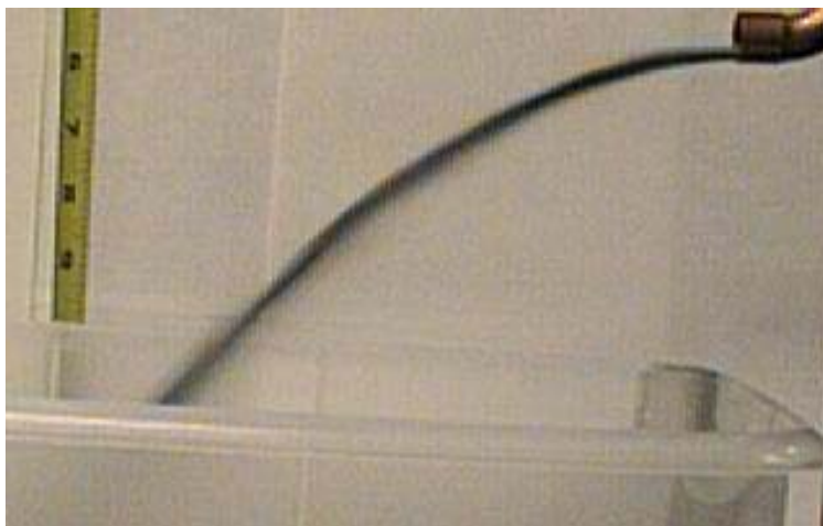
Figure 4: A horizontal jet of 325-mesh tungsten powder after falling 1.5 m inside a 1.25-cm-diameter tube with a 3-cm-radius bend of 90° at its bottom.
