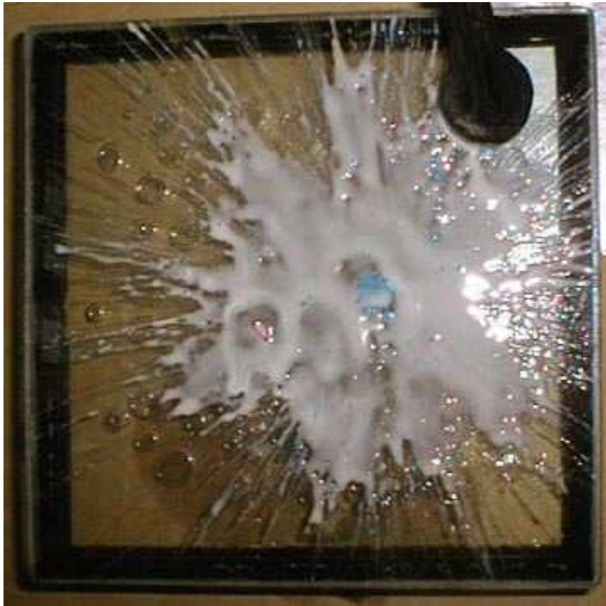
Figure 11: Paintball splat (320 fps) on a 1" glass-lexan laminate from Ballistica, Inc.
