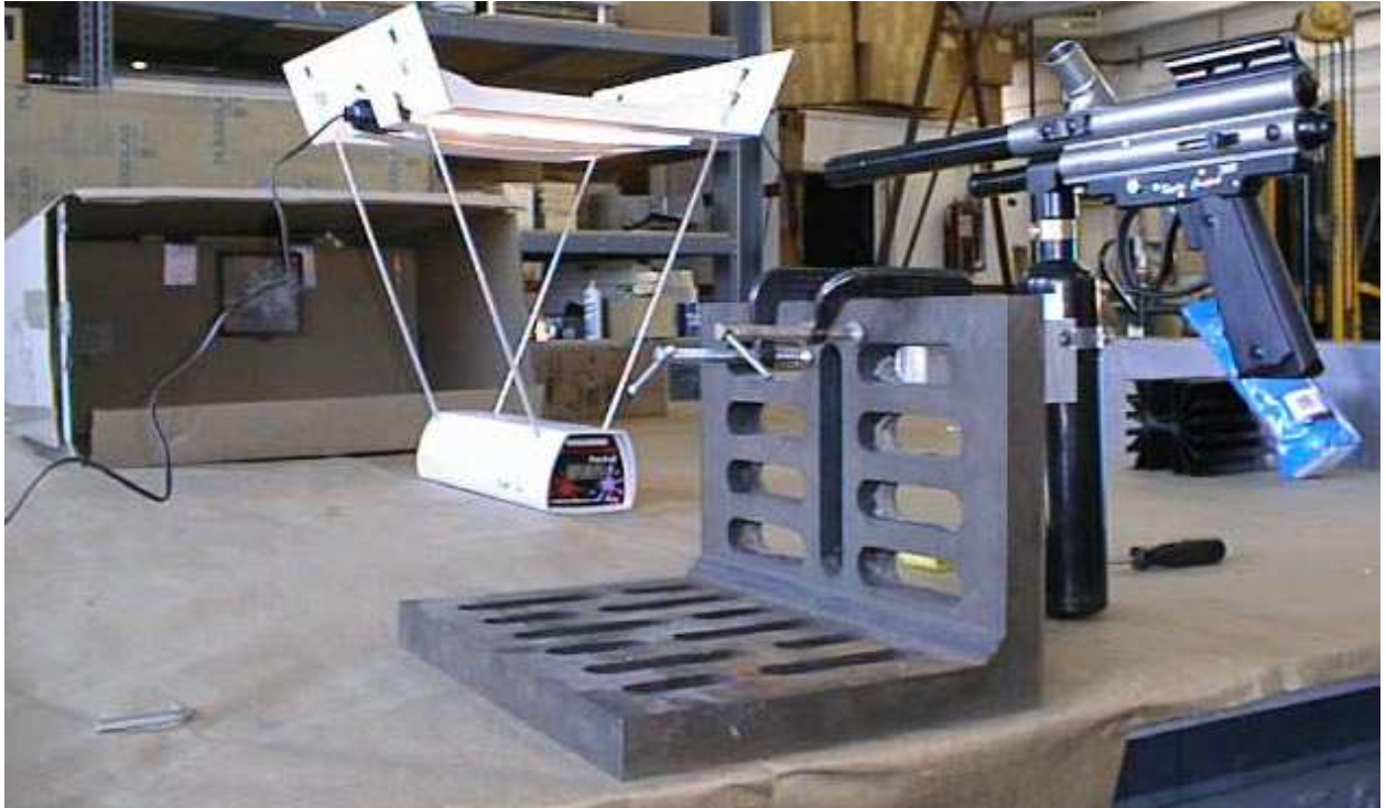
Figure 10: The impact resistance test setup with a Kingman Spyder paintball gun and a Competition Electronics Prochono timer. The distance from the gun to the window under test was about 2 m.
