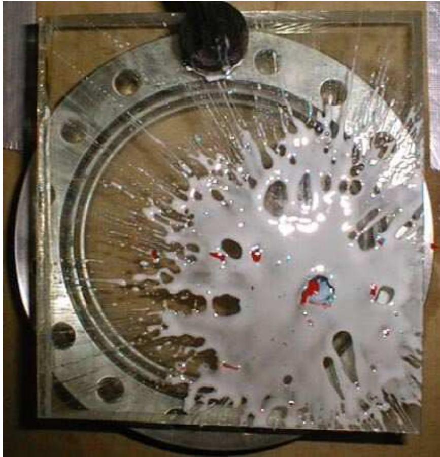
Figure 12: Paintball splat (320 fps) on a 1/4" lexan sheet.
