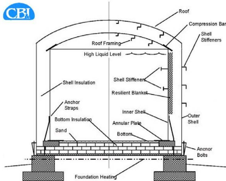
Figure 3: Sketch of a large cryogenic tank designed to contain a liquid-argon TPC (Chicago Bridge and Iron).
