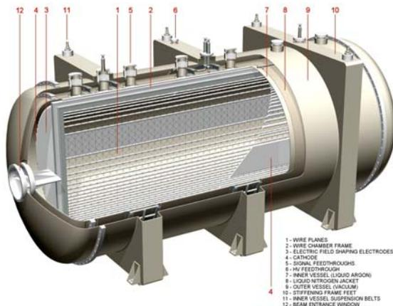
Figure 2: Schematic of cryostat and inner TPC of the  $\sim 100$ -ton prototype [6].
